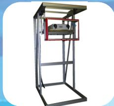
Automatically Retracting Sealer for use above a Gantry Platform
