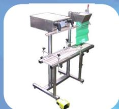
Sealer with Filling Chute and Roller Conveyor for Prepared Foods
