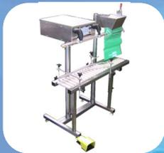
Sealer with Filling Chute and Roller Conveyor for Prepared Foods
