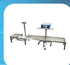
Sealing head over roller conveyor with weighing station
