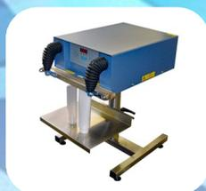
Sealing Head on modified stand for sealing cosmetics tubes
