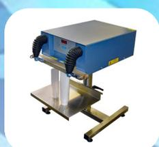
Sealing Head on modified stand for sealing cosmetics tubes
