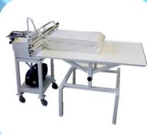
Solenoid Machine with Pneumatic Probe for Faster Vacuum Cycle and Extended Probe Inside Bag
