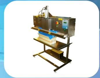
**Vertical Vacuum and Seal Machine for Packing Syringes into Boxes**
