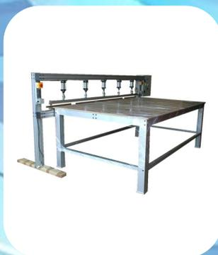
**Gantry Sealer with a Large Work Table for Preparing Composite Materials for Autoclaving**
