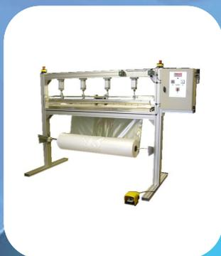
**Gantry Sealer Fitted with a Reel Carrier and Measuring Device for making Pallet Hoods**
